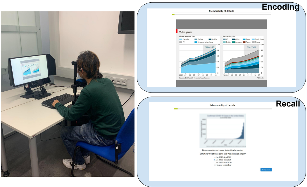
Fig. 4. Left: Recording setup consisting of a high-speed stationary eye tracker, a high-resolution display, and a chin rest. Top: a screenshot of the encoding stage of our study. Bottom: a screenshot of the recall stage of our study.
