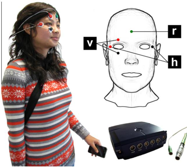
**Fig. 4.** The system we are developing. The image demonstrates the placement of the EOG electrodes on the head and shows the iPhone and the Mobi8 device carried by the user.
